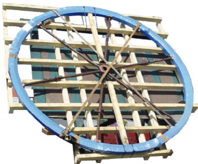
Fig. 9: Stiffening cross for transportation
