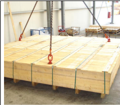
Fig. 4: "Picked crate" on a crane
