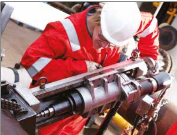
▼ HT40 portable drilling machine.
