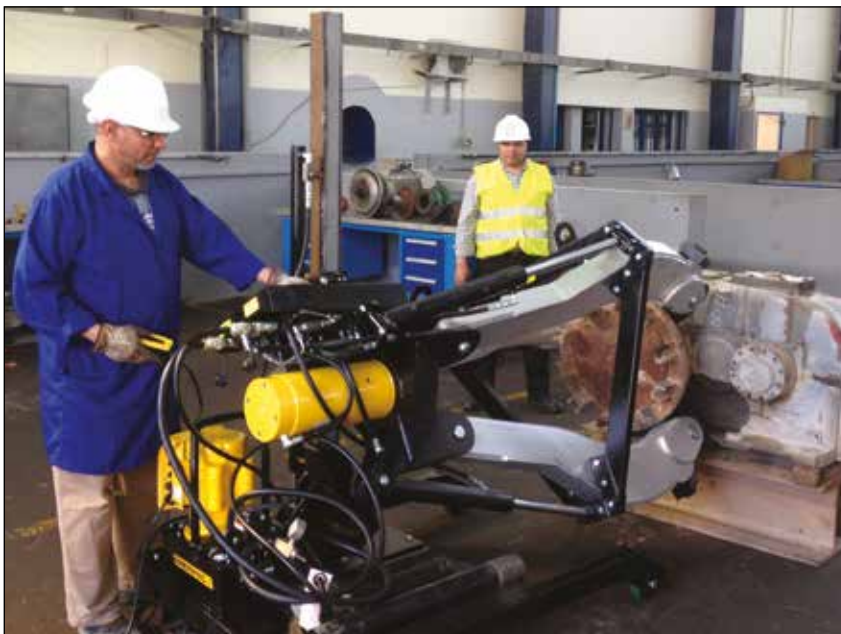
◀ EPH1003E used in maintenance on mining equipment.
