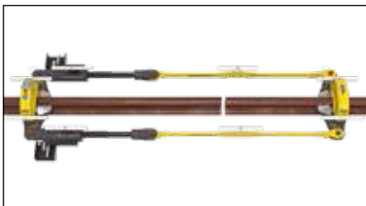
▲ Modular 70 ton stressor and holds the rail in neutral length during the welding process.
