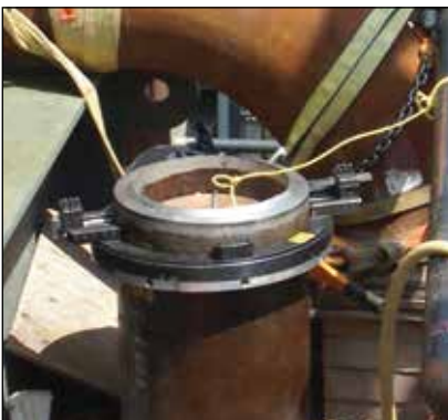
◀ NB-model narrow body clamshell cutter.
