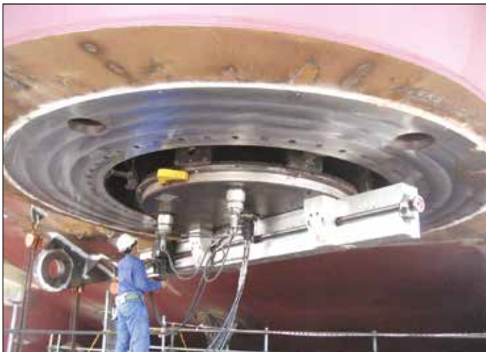
▼ Milling a ship thruster flange.
