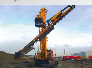
This transport concrete mixer is fitted with a 16.5 m conveyor belt, swivel-mounted in two levels, each having a WD-LC 0419 slew drive
