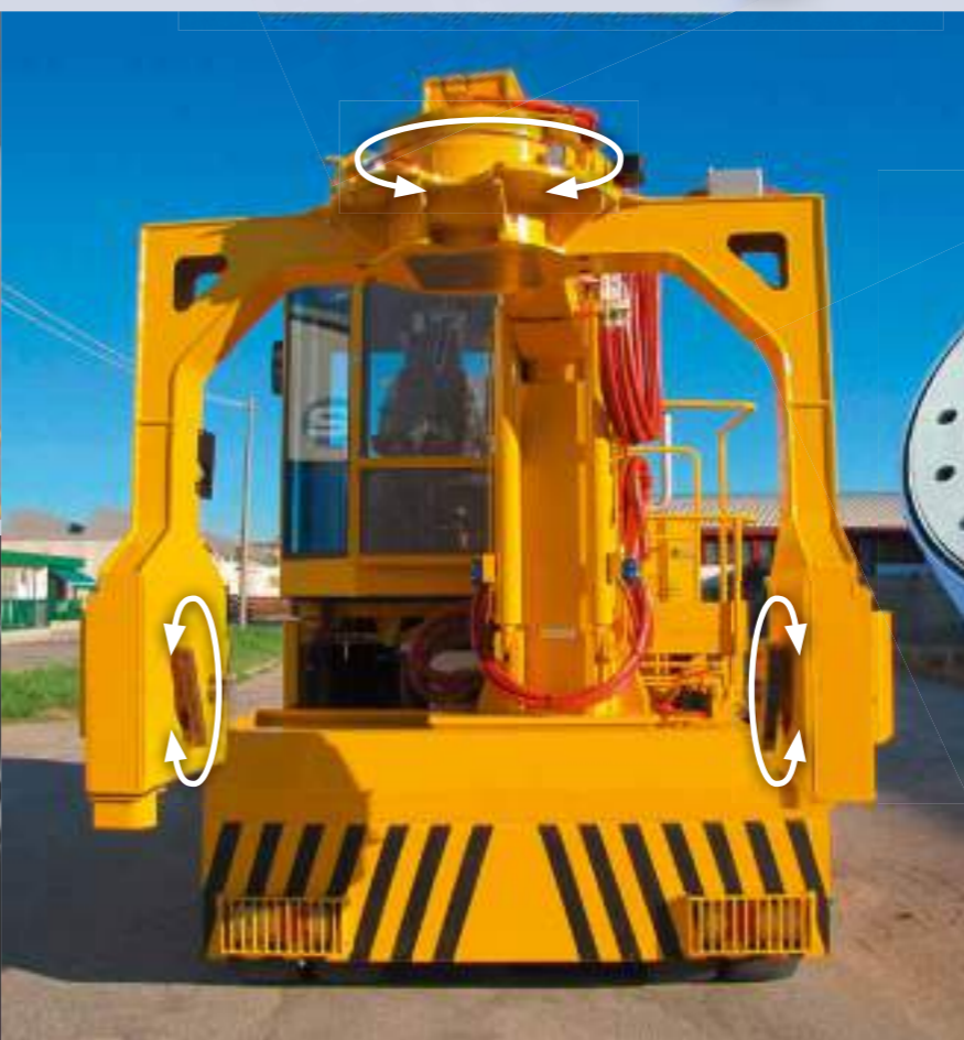
◀ In this transport vehicle for liquid metals , a WD-L slew drive 0478 is installed in the top rotary joint , as well as two additional WD-L slew drives 0343 in the side arms , for slewing the casting ladle .
