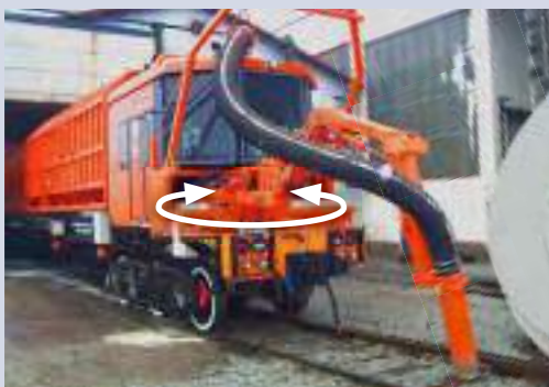
Slew drives of the SP series are integrated in rail vehicles of this type, used to clean tracks.
