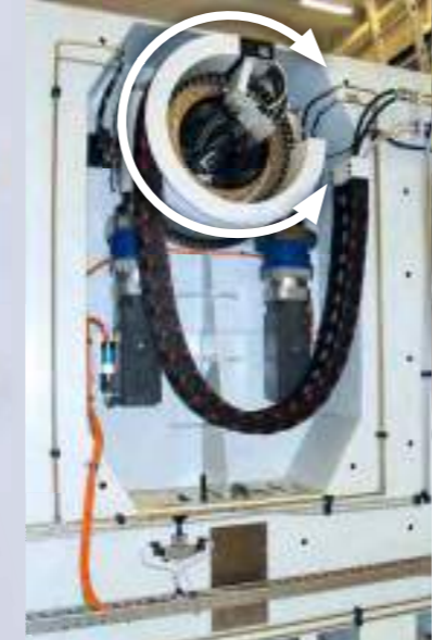
A WD-H 0645 is the central rotation element in this pallet changer for a 5-axis machining center .
