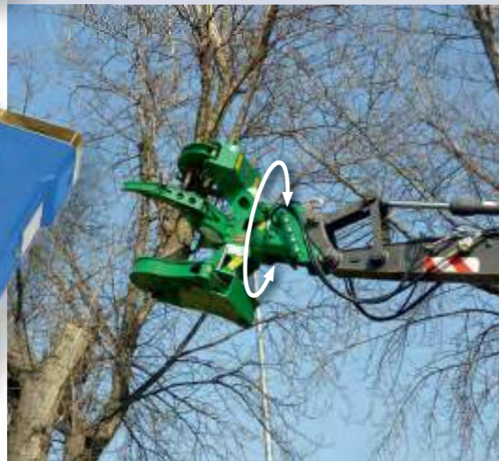
This tree cutter , used to cut back trees and bushes, works using a WD-L 0478 .
