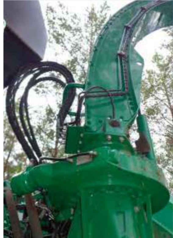
In all the spouts of the wood chippers shown, there is a slew drive of the WD-L series.
