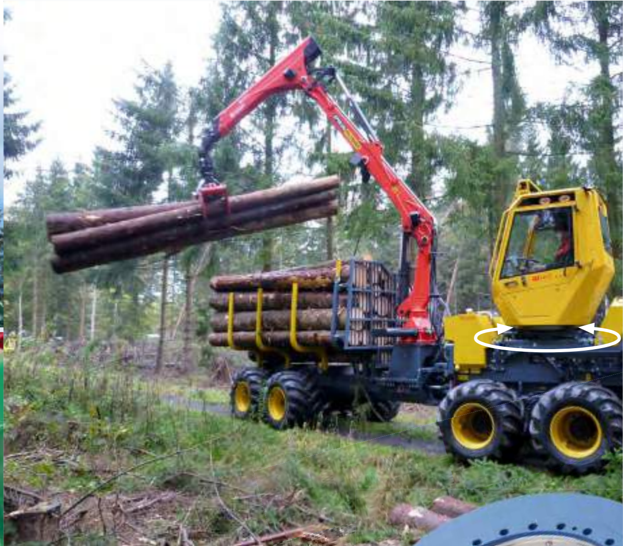
The driver's cab of this combination forestry vehicle is rotated using a slew drive of the SP-I series.
