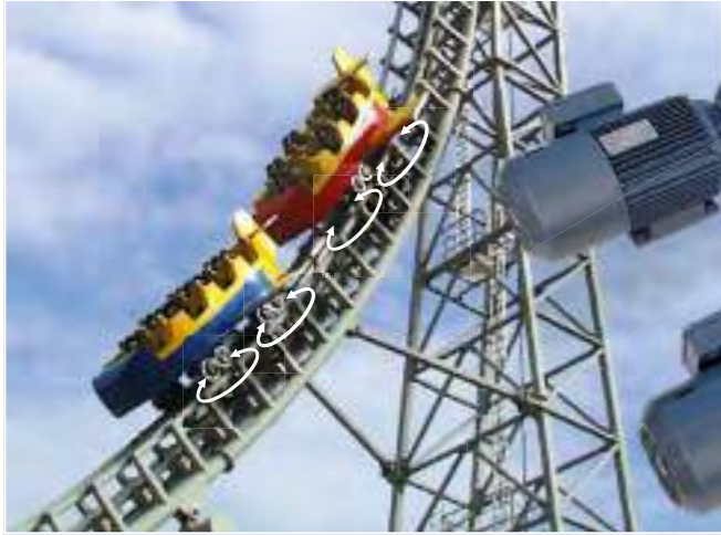
The gondolas of the roller coaster are rotated using a WD-HE 0373 slew drive.
