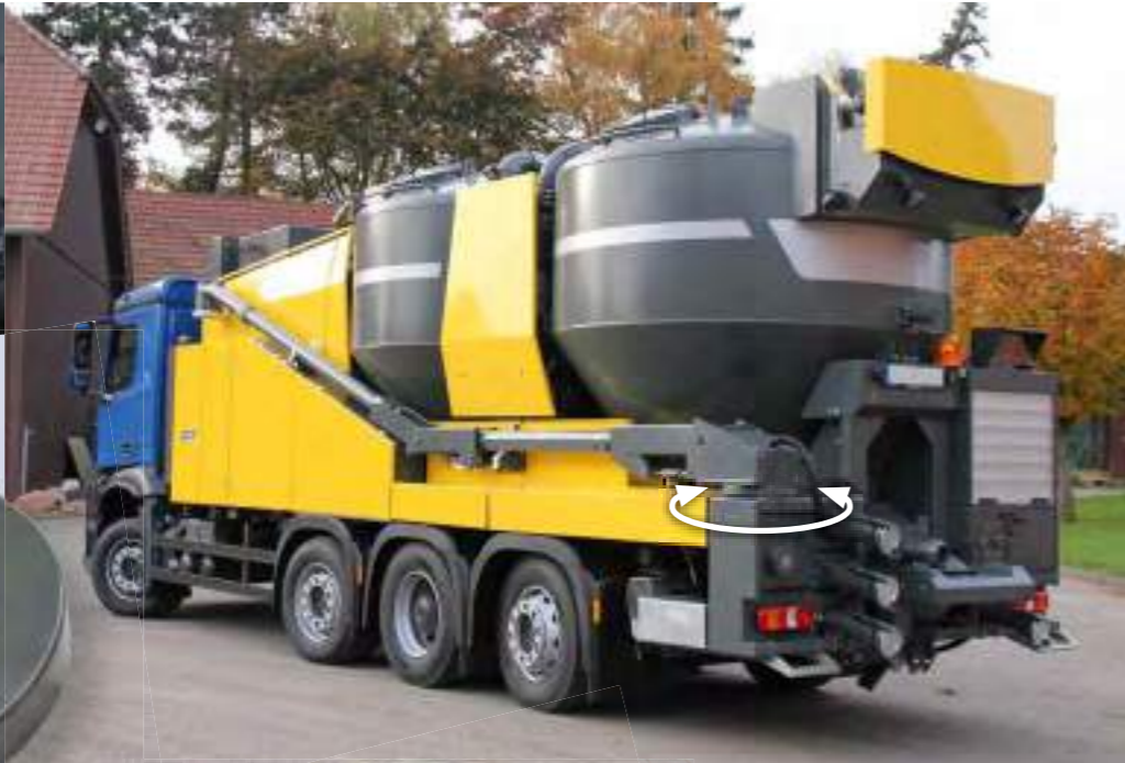
Here, in this high pressure rinsing and suction vehicle , a WD-L 0419 slew drive slews and positions the boom arm for drain cleaning work.
