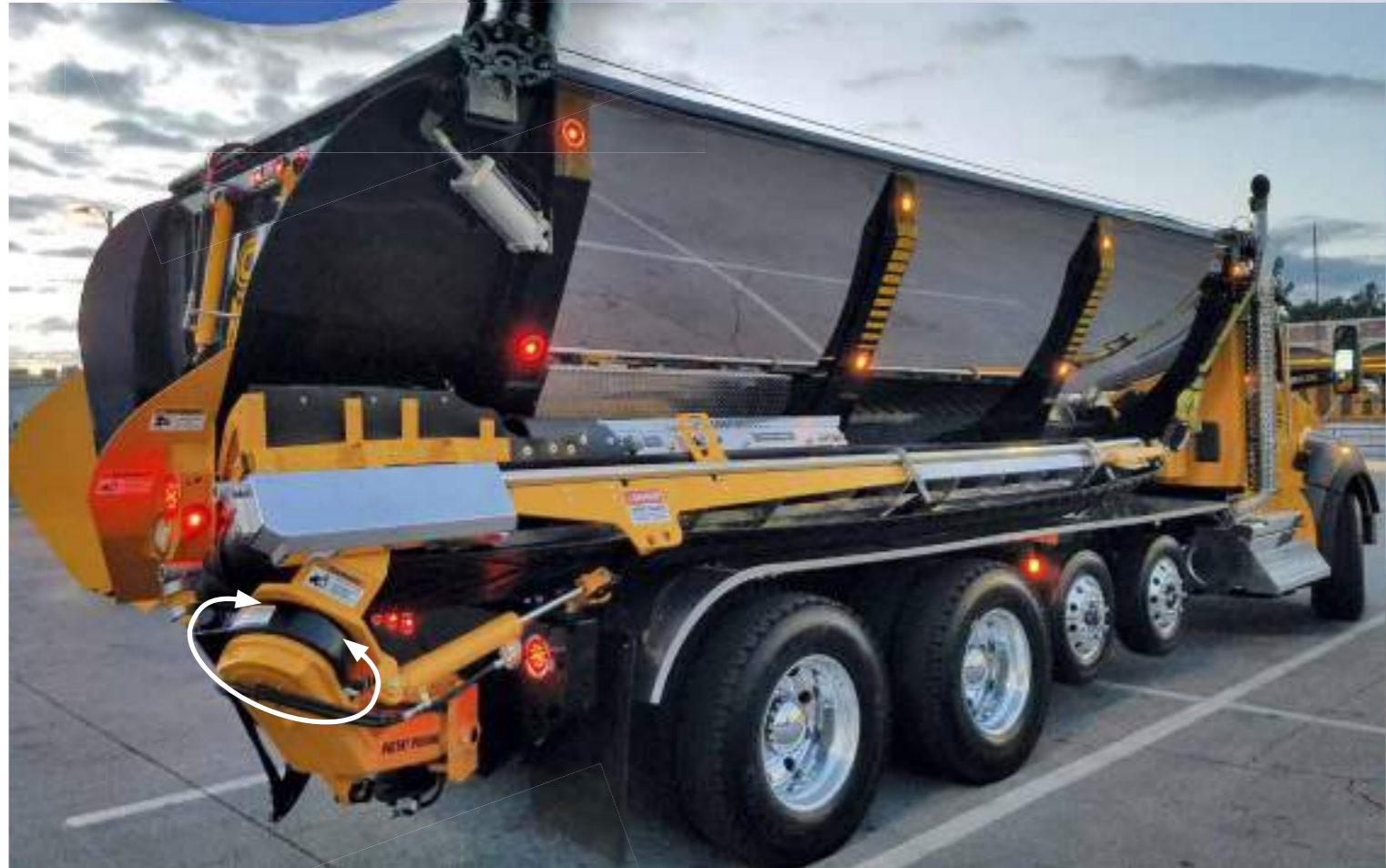
With this special vehicle for bulk material , the discharge is rotated using a WD-L 0343 .
