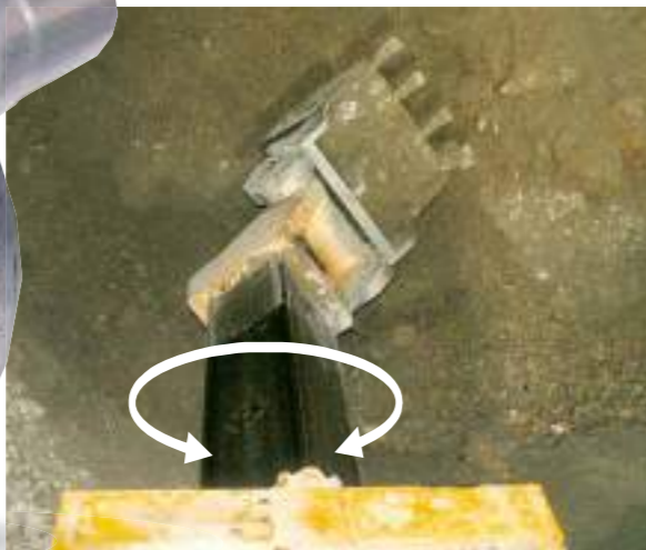
Slew drive SP-HC 0698 with hydraulic gear motors to rotate an excavator arm , which is part of a cutting outrigger of a tunnel boring machine.
