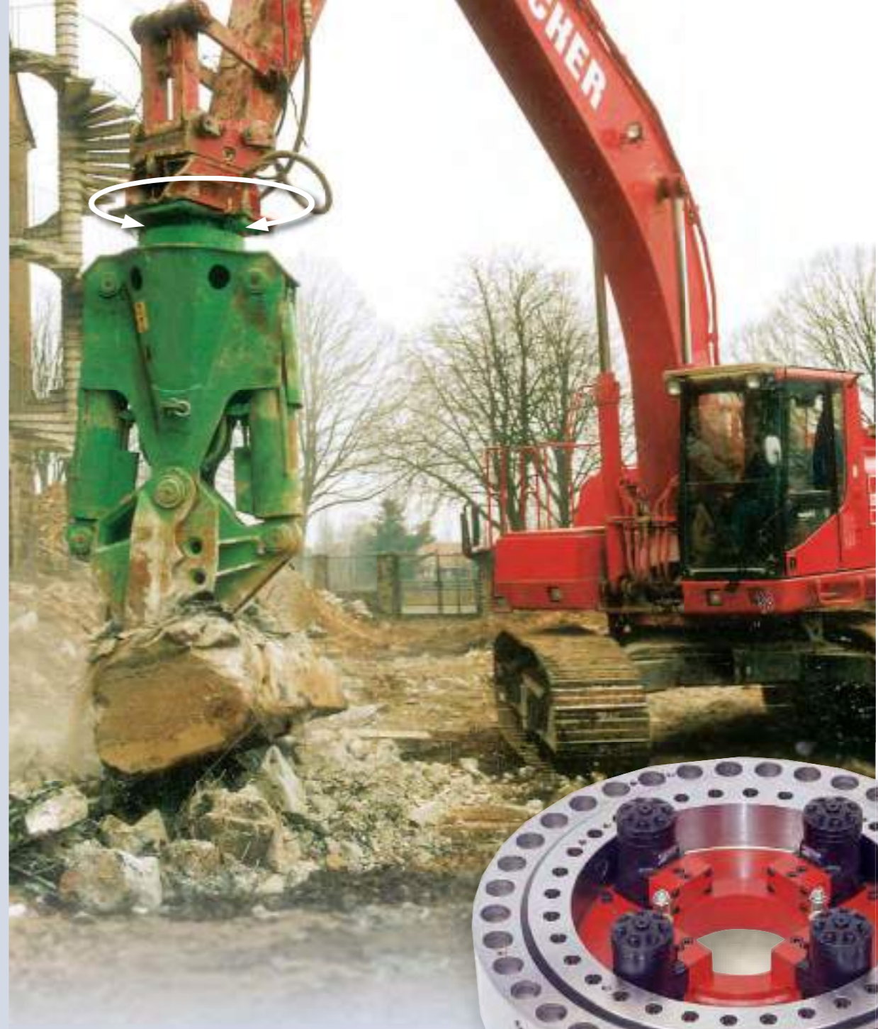
To protect the gear of the slewing device of this concrete demolition pincer safely against damage from overloading, a slip coupling is integrated into the spur gear driven SP-OP 0580 slew drive (OP = "overload protected").
