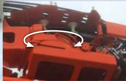
Here, in this high pressure rinsing and suction vehicle , a WD-L 0419 slew drive slews and positions the boom arm for drain cleaning work.
