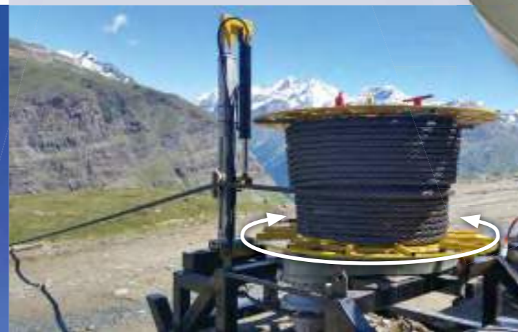
This winch is used in wire rope hoists with tensile forces of up to 3 tonnes. Due to its use at heights of up to 3800 m above sea level , the slew drive of the SP series is exposed to temperatures of -30°C to +20°C .
