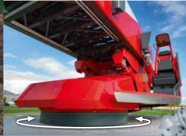
The turntable ladder of this fire truck is rotated using a special slew drive of the SP series .
