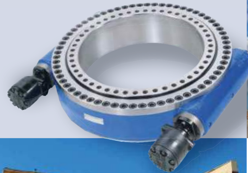
In this ship lift with a width of 22 m and a height of 25 m , there are sixteen axles, each with a WD-H 0645 slew drive. They allow a 360° rotation of each axle.
