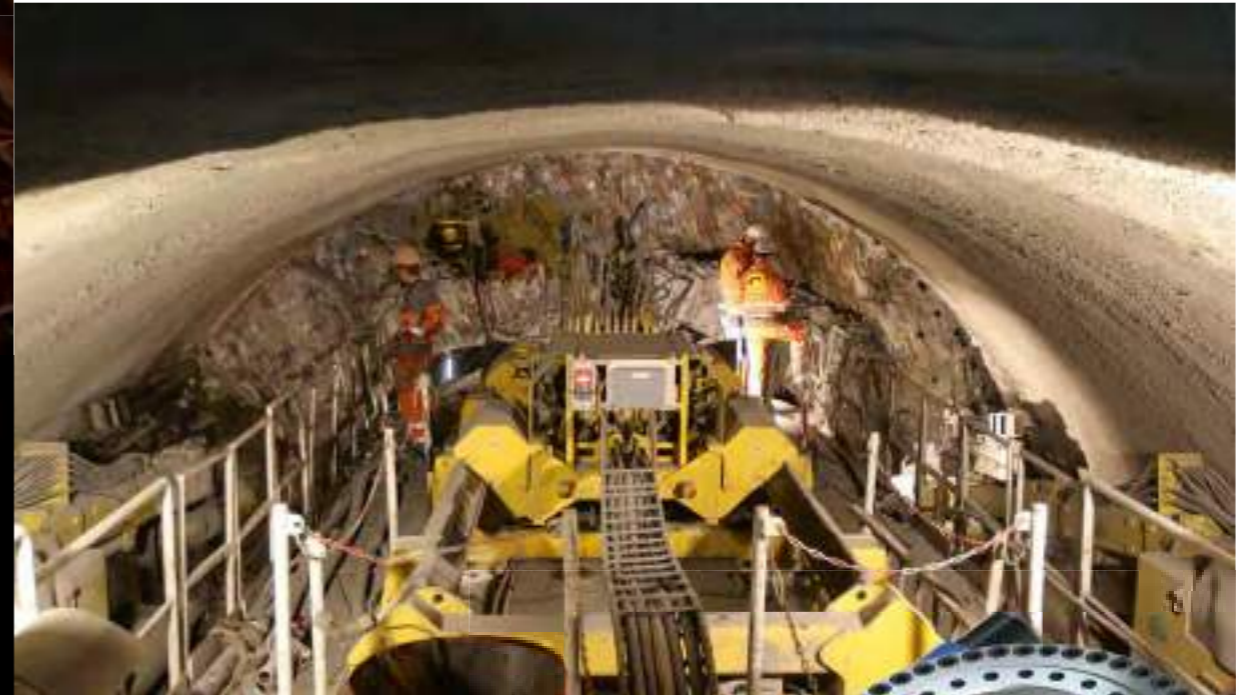
Stone drilling machine, used in deep mining whose drilling device is slewed with a slew drive of the WD-H series.
