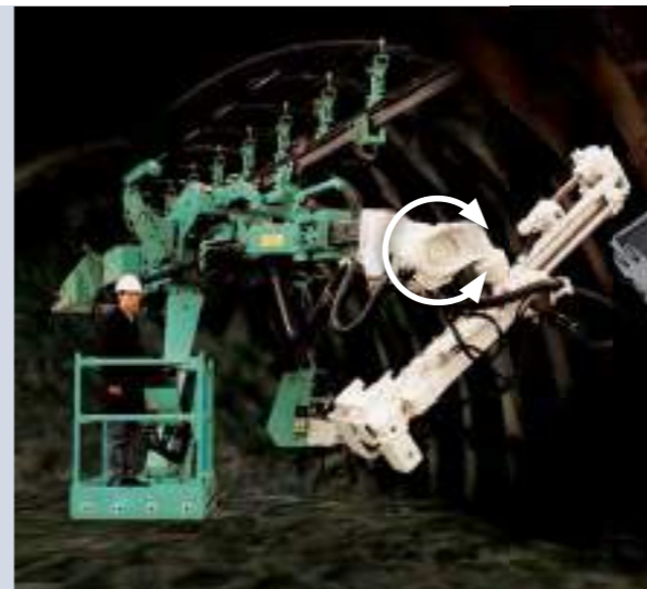
Here, slew drives of the WD-H series are used in a handling grab in deep mining , to maneuver the operating cab of a drilling machine and in a concrete spraying machine to position the long boom.
