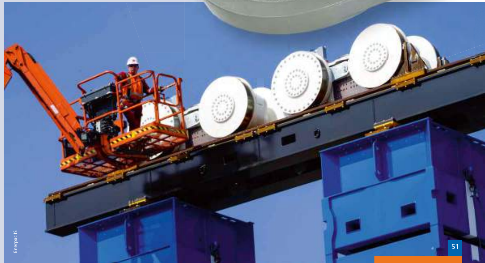
The currently largest traveling crane in the world , with a load capacity of 4,800 tonnes, moves concrete parts for road construction. Each carriage is equipped with 2 SP-HC 0955 slew drives.
