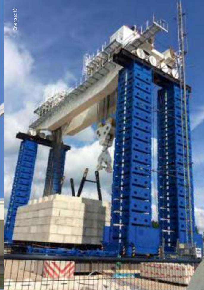
The currently largest traveling crane in the world , with a load capacity of 4,800 tonnes, moves concrete parts for road construction. Each carriage is equipped with 2 SP-HC 0955 slew drives.
