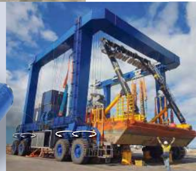
△ This remote-controlled ship lift has a capacity of 320 tonnes. The 16 wheels can be moved in five steering modes: Front wheel, rear wheel and all wheel control, crab steering and carousel operation.
