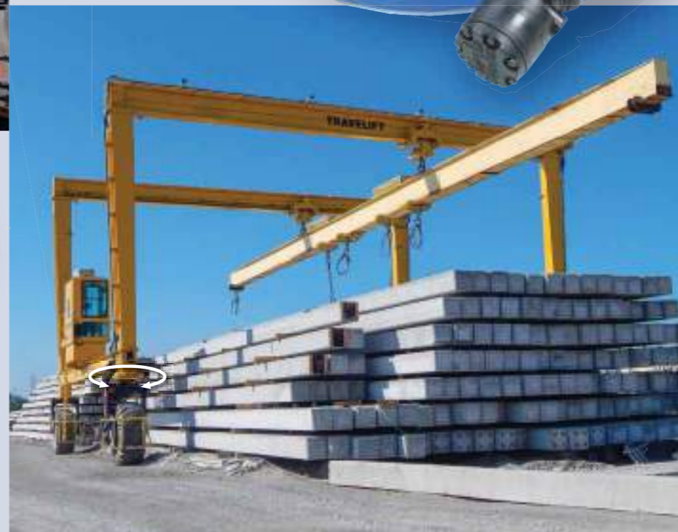
◁ In concrete works, large mobile gantry cranes move heavy, bulky prefabricated concrete parts. The WD-HC 0645 slew drive allows an individual steering angle for all axles. The steering torque under maximum load for stationary steering is approx. 150,000 Nm!
