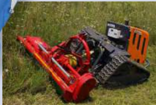
On these slope mowers , the rotational adjustment of the mowing unit or of the motor block is performed by a slew drive of the WD-L series.
