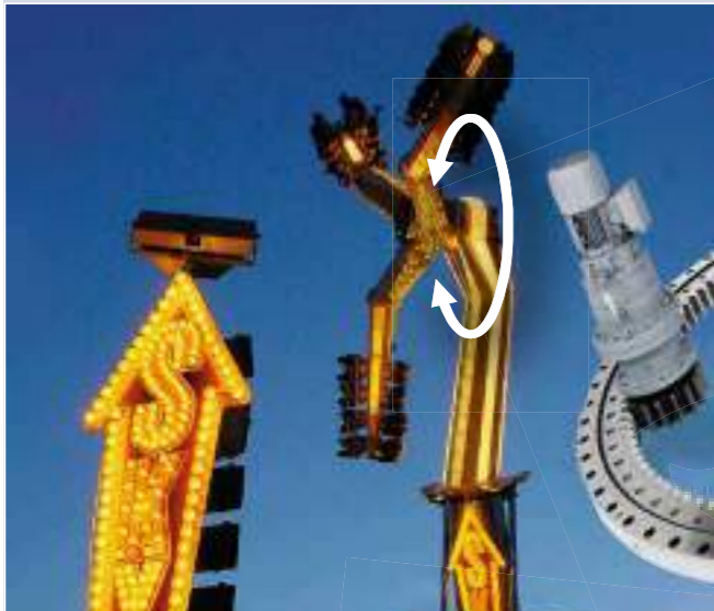
A total of five ball slewing rings with internal gears in three rotation axes are used in this amusement park ride .
