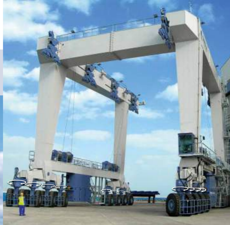
In this ship lift with a width of 22 m and a height of 25 m , there are sixteen axles, each with a WD-H 0645 slew drive. They allow a 360° rotation of each axle.
