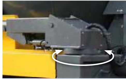
In this mobile animal feed plant , an SP-IC 0229 slew drive is used to rotate the boom.
