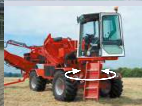
Driver cabs on harvesters can be rotated by a WD-L slew drive with integrated hydraulic motor and permanent brake.
