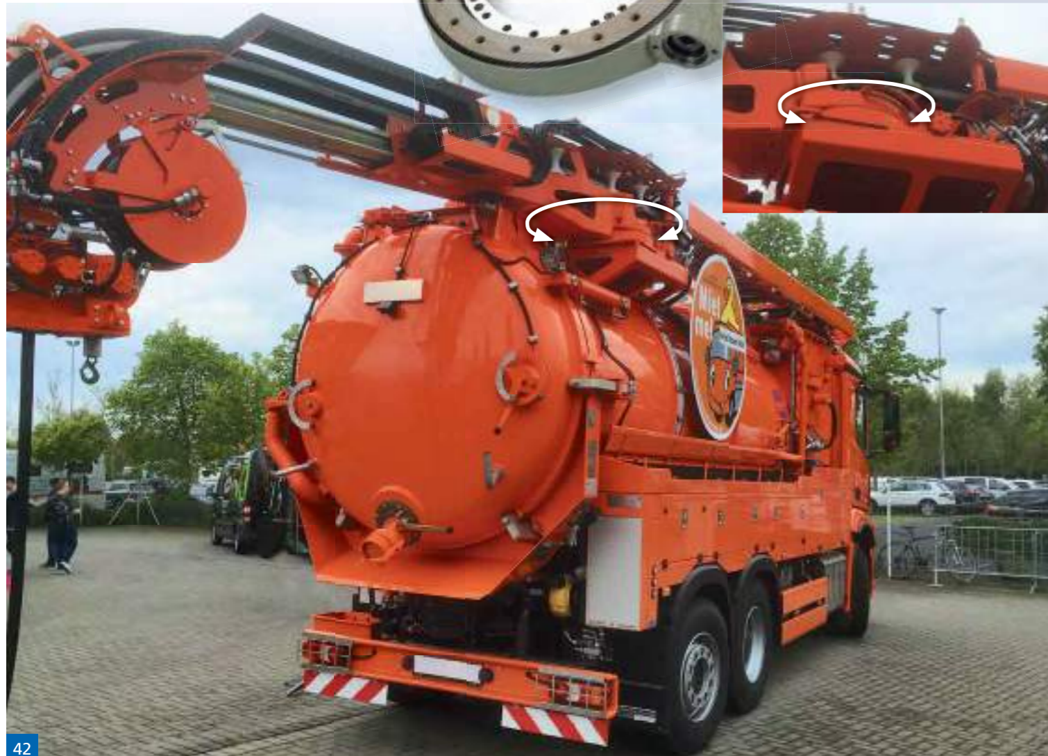
Here, in this high pressure rinsing and suction vehicle , a WD-L 0419 slew drive slews and positions the boom arm for drain cleaning work.
