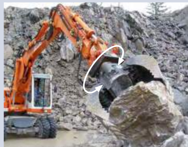
This picker arm is equipped with a slew drive of the SP series as rotary joint.
