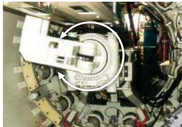
Instead of a standard erector bearing (a geared slewing ring with a large diameter for positioning wall form work for the segment lining of tunnels), this manipulator uses a considerably more compact WD-HC 0373 slew drive with two worms and holding brakes.
