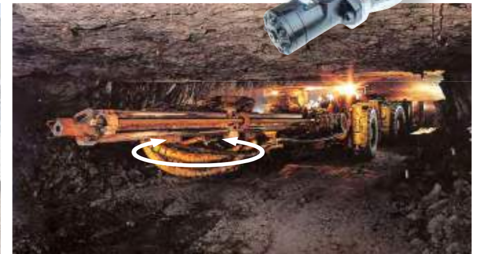
The WD-HC 0220 slew drive shown here has an integrated locking device with decouplable spur gear to secure the position of this deep mining blast hole drilling rig , during drilling.
