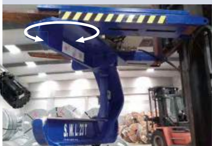
WD-L slew drives are used in these forklift rotators .
