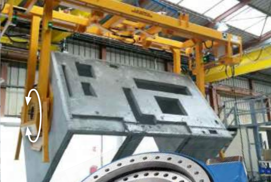
◀ A positioning and slewing device in combination with a hall crane for heavy machine elements and workpieces. Here, size 0478 WD-L slew drives are in use.
