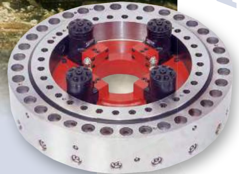
To protect the gear of the slewing device of this concrete demolition pincer safely against damage from overloading, a slip coupling is integrated into the spur gear driven SP-OP 0580 slew drive (OP = "overload protected").
