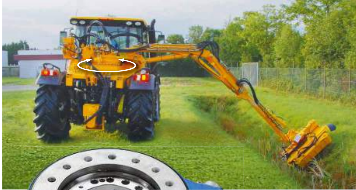
On these slope mowers , the rotational adjustment of the mowing unit or of the motor block is performed by a slew drive of the WD-L series.
