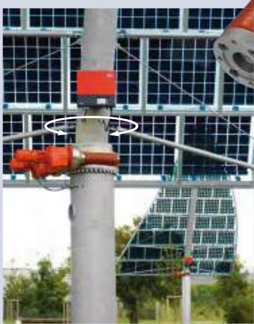
Solar trackers , which track the sun using slew drives of the WD-L and WD-H series.
