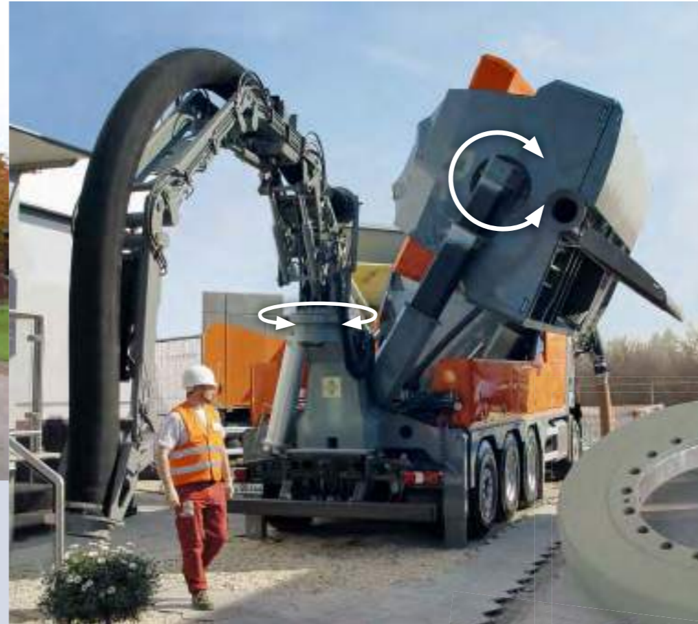
3 slew drives are used in this suction dredger : A WD-LC 0625 to rotate/tip out the grouped goods container, a WD-L 0419 to slew the entire suction boom and an SP-I 0311 to rotate a front, geared pipe for loosening stones and earth.
