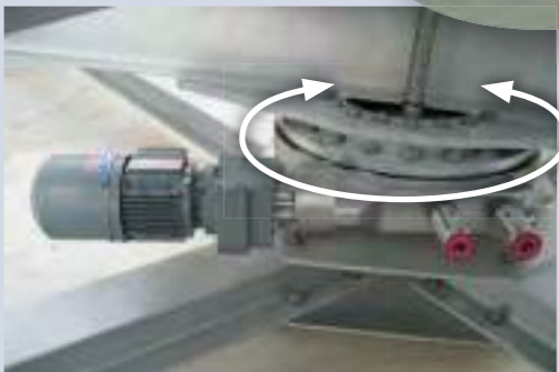
On-roof plant trackers can be rotated with slew drives (here, a slew drive of the WD-L series is used).
