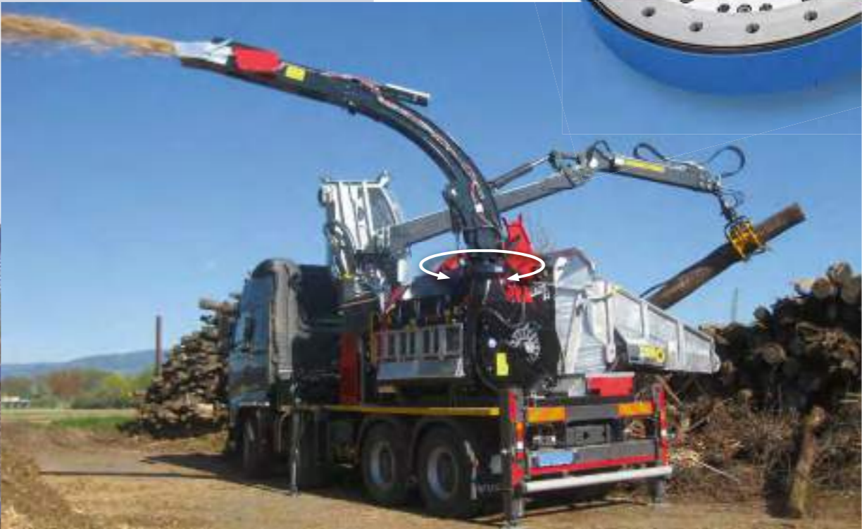
These chippers are equipped with slew drives of the WD-L and SP-I series, to position the chipper and/or the spout.
