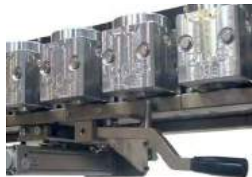
Detail of the manual tool loading/unloading station
