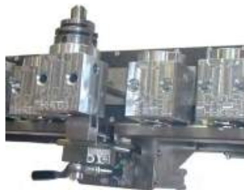
Detail of the tool change extraction station
