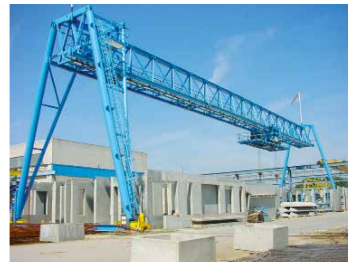
Gantry crane with rotatable loading device in a concrete factory.
