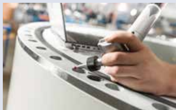
Inspection of a roller bearing by means of 3D measurement equipment
