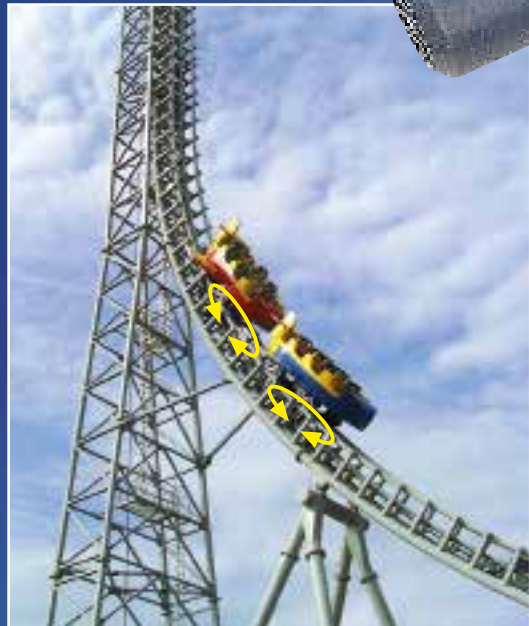
A ride in "Zero g" guarantees thrills and also zero gravity for a short time. The gondolas are rotated with our Slew Drive WD-HE 0373.
