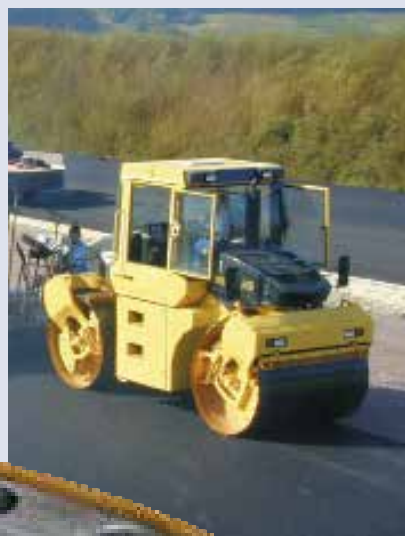
Tandem asphalt compaction rollers use untoothed Slewing Rings as a steering bearing (some designs are partly coated on the surface to prevent corrosion). In the split roller, Slewing Rings with special seals are used.
