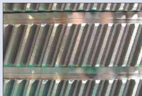
External helical gear, normalized
