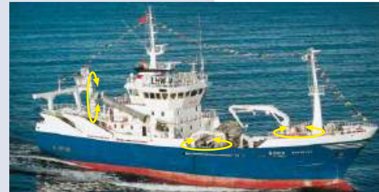
Deep sea fishing vessels use Ball Slewing Rings for shipboard cranes and net handling equipment. Typical external diameters range between 600 to 1,500 mm (23,6 to 59 in).
