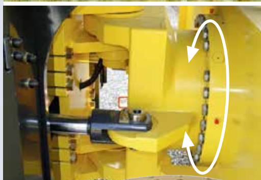
The vibratory roller of the refuse compactor in the picture uses untoothed Slewing Rings in the knuckle joint.
