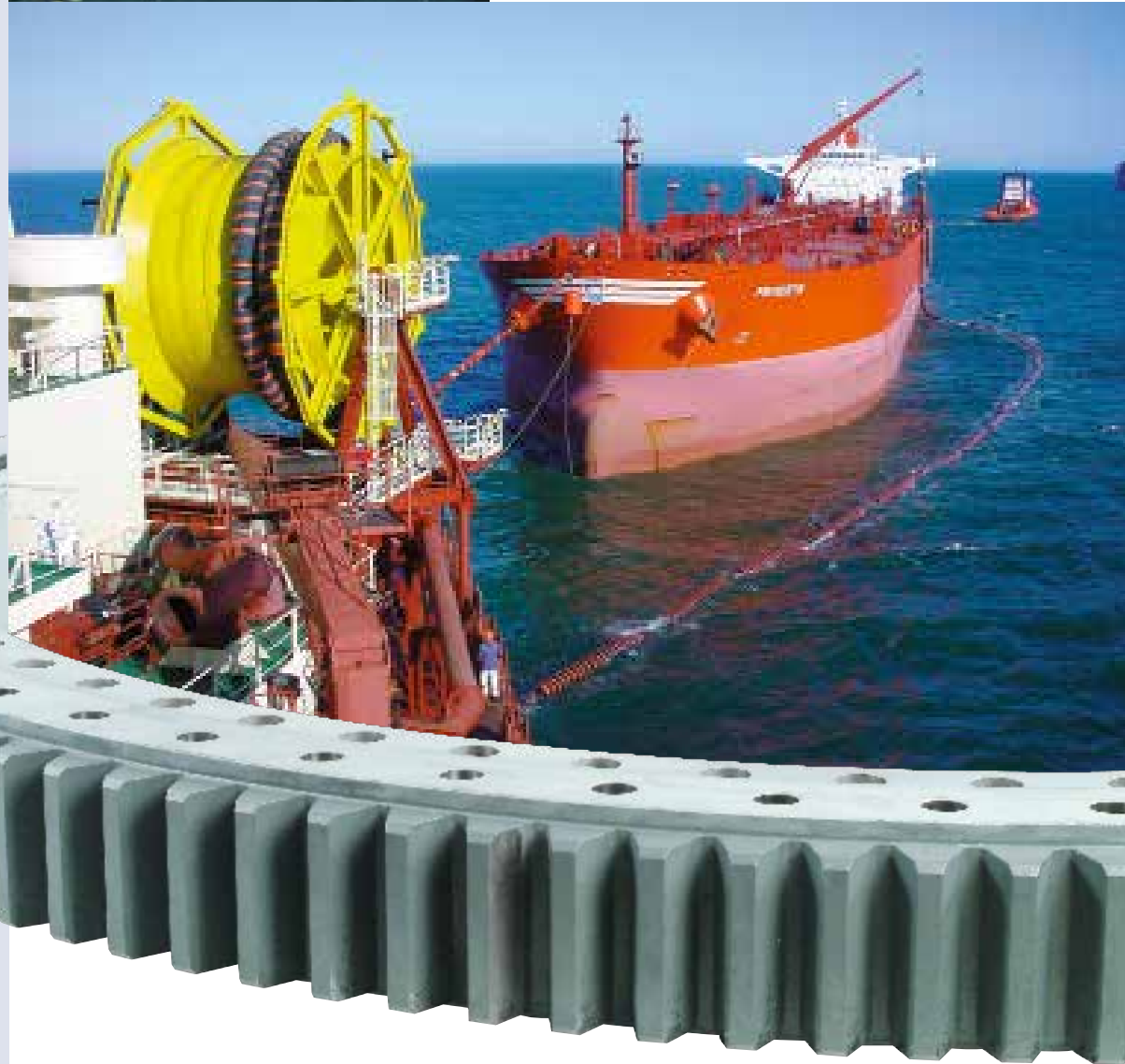
External toothed Ball Slewing Rings with a diameter of 3,000 mm (118 in) are used in this oil spill barrier reel on an FPSO (Floating Production Storage Offloading) unit.
