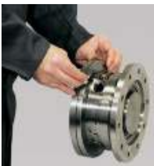
3 Remove sealing plug from injector connection.
