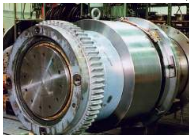
1 HYGUARD® Safety coupling/brake disk combination in a four-high stand, built-in between main motor and pinion stand gearbox.
