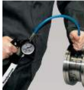
4 Connect pump, loosen shear tube by 1/4 turn.
