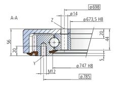
The mounting structure must support the housing to at least ø741.
