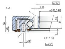
The mounting structure must support the housing to at least ø411.
