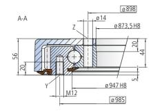
The mounting structure must support the housing to at least ø941.
