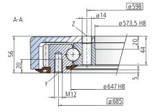
The mounting structure must support the housing to at least ø641.
